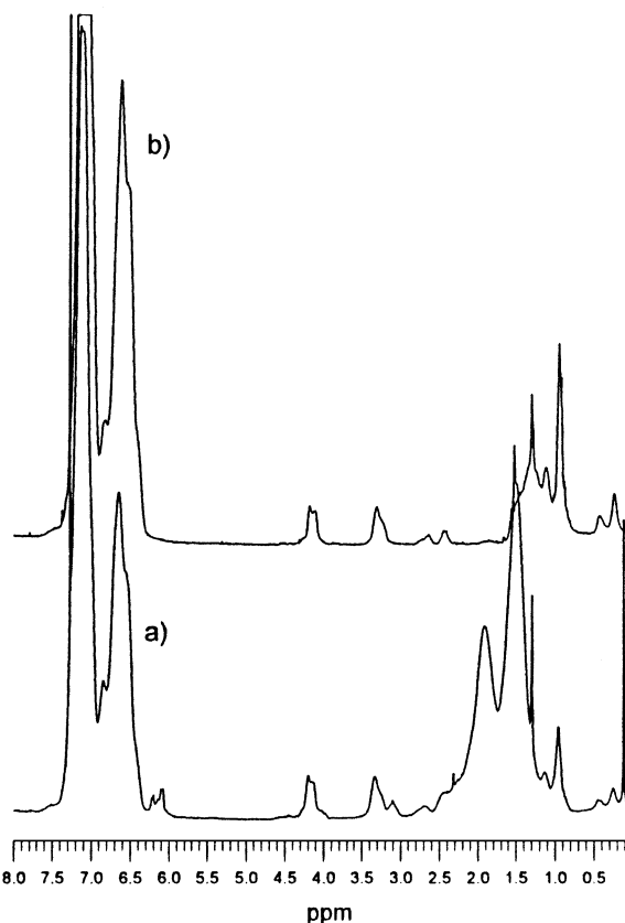
Fig. 1. (a) ^1\text{H} NMR spectrum (200 MHz, \text{CDCl}_3 ) of P1; (b) ^1\text{H} NMR spectrum (200 MHz, \text{CDCl}_3 ) of partially deuterated P1.
